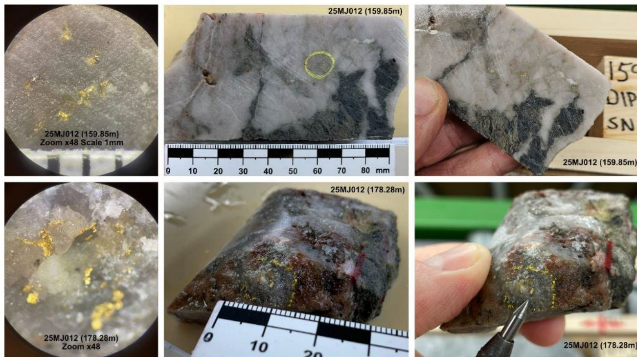
Figure 21: Examples of the visible gold in 25MJ012 within quartz veins at 159.9m and 178.3m downhole.
